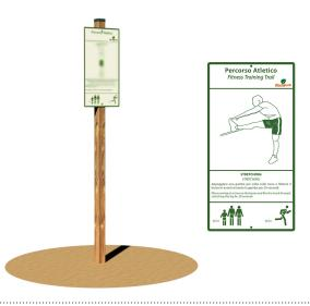
POLE MOUNTED PANEL **To be matched to the Stretching fitness trail station - Art. 2127** Aluminium Dibond® panel 62x33 cm, 3 mm thick, that shows how to properly perform the exercise and the number of repetitions. The panel is supported by a pole made of glued laminated pine timber pressure treated with non-toxic salts, section 7x7 cm and 250 cm height, for ground anchoring system.
