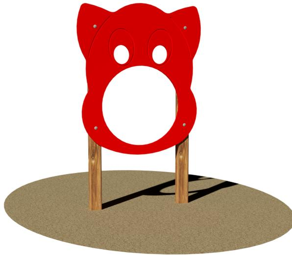
DogStructure made of Nordic Pine wood pressure treated with non-toxic salts. Components: 2 glued laminated pine timber poles section cm 7x7 assembled to a coloured polyethylene panel PEHD without sharp edges mm 15 thick. Assembly system with 8.8 galvanized steel bolts and self-locking nuts. Coloured nylon cap nuts as required by law. Pole caps in polyethylene.
