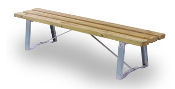
The structure consists of 2 hot galvanized tubular steel supports with a "U" section, 190 cm in length. The seat is composed of three Nordic Pine wood planks pressure treated with non-toxic salts, section 110 x 45 mm and fixed through galvanized steel bolts. Anchorage system: to be fixed on the ground. Supplied in an assembly-kit.
