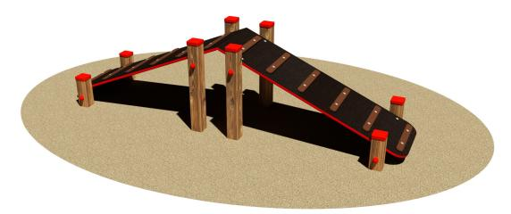
Structure made of Nordic Pine wood pressure treated with non-toxic salts. Components: N°2 platforms in multi-layer birch wood glued with phenol formaldehyde resin with non-slip knurled surface and finished with a coloured overlay film in both sides. The platforms are supported by N°4 glued laminated pine timber poles section cm 7x7. Assembly system with 8.8 galvanized steel bolts and self- locking nuts. Coloured nylon cap nuts as required by law. Pole caps in polyethylene.
