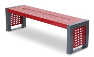
The structure consists of 2 tubular supports with a square section 70 x 70 mm and side panels in perforated metal sheet (square hole). Seat made of steel folded under pressure 30/10 thick with square holes, fixed to the supports through galvanized steel bolts. Anchorage system: to be fixed on the ground. Supplied in an assembly-kit. Metal structure entirely galvanized and baked finishing at 180°C.
