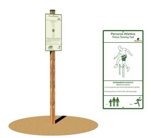
POLE MOUNTED PANEL **To be matched to the Obstacles course fitness trail station - Art. 2117** Aluminium Dibond® panel 62x33 cm, 3 mm thick, that shows how to properly perform the exercise and the number of repetitions. The panel is supported by a pole made of glued laminated pine timber pressure treated with non-toxic salts, section 7x7 cm and 250 cm height, for ground anchoring system.
