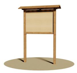
Made of northern pine impregnated in autoclave with non-toxic salts. Composed of two uprights sect. cm 9 x 9 and a frame containing the central panel in mahogany okoumé, phenolic glueing and finished with transparent wax paintings. Match boarding two-pitch roof. Assembly through galvanized 8.8 screw bolts and locknuts. nut-caps in coloured nylonaccording to the standard.
