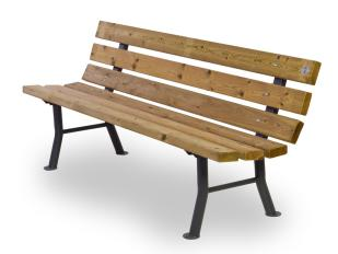
The structure consists of 2 tubular painted galvanized steel supports Ø 50 mm and U shape profiles. The seat and the backrest consist of six Nordic Pine wood planks pressure treated with non-toxic salts, section 110 x 45 mm and 190 cm length. Galvanized steel bolts. Supplied in an assembly-kit. Powder coating at 180°C. Anchorage system: to be fixed on the ground.
