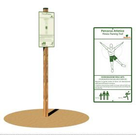
BODYWEIGHT WORKOUT WITHOUT ANY EQUIPMENT Aluminium Dibond® panel 62x33 cm, 3 mm thick, that shows how to properly perform the exercise and the number of repetitions. The panel is supported by a pole made of glued laminated pine timber pressure treated with non-toxic salts, section 7x7 cm and 250 cm height. Assembly system with 8.8 galvanized steel bolts and self- locking nuts. Coloured nylon cap nuts as required by law. Polyethylene post caps. Ground anchoring system.
