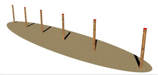
Dog Agility weave poles. Structure made of glued laminated pine timber pressure treated with non-toxic salts. Components: 6 vertical poles placed in a row at an appropriate distance. Assembly system with 8.8 galvanized steel bolts and self- locking nuts. Coloured nylon cap nuts as required by law. Pole caps in polyethylene. Overall dimensions: cm 950 x 7 x 120 h
