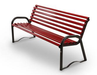
Bologna Bench. Street furniture. The structure consists of 2 tubular steel supports Ø 40 mm, with an anatomical shape and with armrests, 158 cm in length. It consists of twelve steel bars with an oval section 40x20 mm equipped with plastic caps at both ends. Fastening system to the supports through galvanized steel bolts. Anchorage system: to be fixed on the ground. Supplied in an assembly-kit. Entirely galvanized, baked finishing at 180°C.
