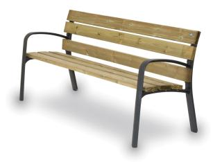
Alicia Wood Bench 180 Pine. Pine wood bench 180. Bench with two cast iron supports and six pine wood planks section 110 x 33 mm and galvanized burnished steel bolts. Treatment of the wood with special water-repellent preservatives in order to provide full protection against fungal growth. Treatment of the supports with anti-rust primer and baked finishing at 180°C. Anchorage system: to be fixed on the ground.
