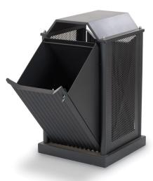
Malta outdoor litter bin. Main structure made of tubular steel, for ground anchoring system. It is equipped with a roof top made of pressed steel sheet, fixed to the structure through 4 stainless steel bolts. Side panels in pressed perforated steel sheet with reinforced edges. Basket in steel sheet with small inner crossbars for attaching the waste bag. Emptying system by unhooking and tilting through hinges. Locking system with key (supplied). Fully galvanized. Powder coating at 180°C.
