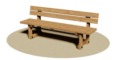
Made of northern pine impregnated in autoclave with non-toxic salts. Length cm.190. Structure composed by two assembled supports in rectangular section wood. Back composed by two boards section mm 110x45. Seat composed by 4 boards section mm 90x45. Everything is assembled by zinc plated steel bolts. The bench is supplied with an assembly kit. Weight kg 34; Seat height cm 48.
