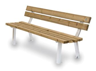
Anatomica bench. Nordic Pine wood bench. The structure consists of 2 hot galvanized tubular steel supports with a "U" section and Nordic Pine wood pressure treated with non-toxic salts; 190 cm length. The backrest is composed of two planks section 110 x 45 mm fixed through galvanized steel bolts and a seat made of four planks section 90 x 45 mm both fixed through galvanized steel bolts. Anchorage system: to be fixed on the ground. Supplied in an assembly-kit.
