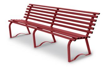
The structure consists of 3 tubular steel supports with a square section 30 x 30 mm with an anatomical shape, 200 cm in length. It consists of twelve steel bars with an oval section 40x20 mm equipped with plastic caps at both ends. Fastening system to the supports through galvanized steel bolts. Anchorage system: to be fixed on the ground. Supplied in an assembly-kit. Entirely galvanized, powder coating at 180°C.
