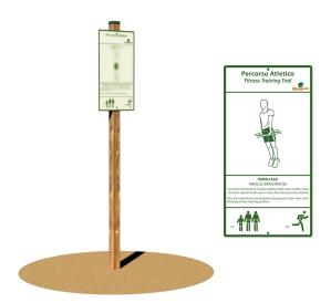
POLE MOUNTED PANEL **To be matched to the Parallel bars exercise fitness trail station - Art. 2119** Aluminium Dibond® panel 62x33 cm, 3 mm thick, that shows how to properly perform the exercise and the number of repetitions. The panel is supported by a pole made of glued laminated pine timber pressure treated with non-toxic salts, section 7x7 cm and 250 cm height, for ground anchoring system.
