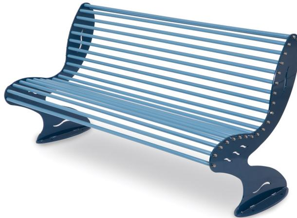
Ghost Bench (RAL 5024-5001). Modern bench. The structure consists of 2 supports in steel sheet 8 mm thick, with an anatomical shape. The seat and the backrest are composed of 21 tubular steel bars  $\varnothing$  20 mm. Fastening system to the supports through stainless steel bolts. Anchorage system: to be fixed on the ground. Supplied in an assembly-kit. Entirely galvanized, baked finishing at 180°C.
