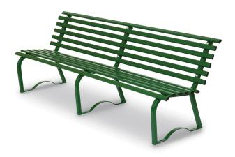
The structure consists of 3 tubular steel supports with a square section 30 x 30 mm with an anatomical shape, 200 cm in length. It consists of twelve steel bars with an oval section 40x20 mm equipped with plastic caps at both ends. Fastening system to the supports through galvanized steel bolts. Anchorage system: to be fixed on the ground. Supplied in an assembly-kit. Entirely galvanized, powder coating at 180°C.
