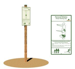
BODYWEIGHT WORKOUT WITHOUT ANY EQUIPMENT Aluminium Dibond® panel 62x33 cm, 3 mm thick, that shows how to properly perform the exercise and the number of repetitions. The panel is supported by a pole made of glued laminated pine timber pressure treated with non-toxic salts, section 7x7 cm and 250 cm height. Assembly system with 8.8 galvanized steel bolts and self- locking nuts. Coloured nylon cap nuts as required by law. Polyethylene post caps. Ground anchoring system.
