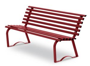
The structure consists of 2 tubular steel supports with a square section  $30 \times 30$  mm with an anatomical shape, 150 cm in length. It consists of twelve steel bars with an oval section 40x20 mm equipped with plastic caps at both ends. Fastening system to the supports through galvanized steel bolts. Anchorage system: to be fixed on the ground. Supplied in an assembly-kit. Entirely galvanized, powder coating at  $180^{\circ}$ C.
