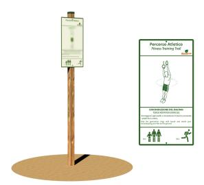
POLE MOUNTED PANEL **To be matched to the Torso rotation exercise fitness trail station - Art. 2133** Aluminium Dibond® panel 62x33 cm, 3 mm thick, that shows how to properly perform the exercise and the number of repetitions. The panel is supported by a pole made of glued laminated pine timber pressure treated with non-toxic salts, section 7x7 cm and 250 cm height for ground anchoring system.
