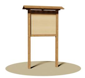
Made of northern pine impregnated in autoclave with non-toxic salts. Composed of two uprights sect. cm 9 x 9 and a frame containing the central panel in mahogany okoumé, phenolic glueing and finished with transparent wax paintings. Match boarding two-pitch roof. Assembly through galvanized 8.8 screw bolts and locknuts. nut-caps in coloured nylonaccording to the standard.
