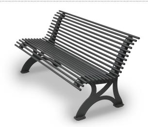
Armonia bench. Outdoor Steel Bench. The structure consists of 2 supports in galvanized steel sheet 8 mm thick, with an anatomical shape; 150 cm length. No.22 round steel tubes Ø20 mm, each equipped with plastic caps on either end. Fastening system to the supports through galvanized steel bolts. Anchorage system: to be fixed on the ground. Supplied in an assembly-kit. Colour: micaceous dark grey. Entirely galvanized and baked finishing at 180°C. Supplied in an assembly-kit.
