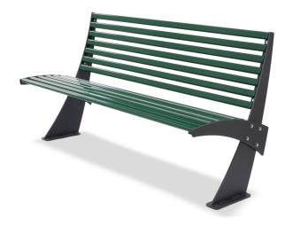
Contemporary bench for street furniture. The structure consists of 2 supports in steel sheet 8 mm thick, with an anatomical shape. The seat and the backrest are composed of 2 units which consist of seven tubular steel bars each with an oval section 40x20 mm. Fastening system to the supports through galvanized steel bolts. Anchorage system: to be fixed on the ground. Supplied in an assembly-kit. Entirely galvanized, baked finishing at 180°C.
