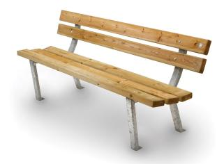
Bosco Bench. The structure consists of 2 hot galvanized tubular steel supports with a "U" section, 190 cm in length. The backrest and the seat are composed of five Nordic Pine wood planks pressure treated with non-toxic salts, section 110 x 45 mm and fixed through galvanized steel bolts. Anchorage system: to be fixed on the ground. Supplied in an assembly-kit.
