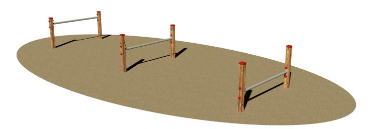
Structure made of glued laminated pine timber pressure treated with non-toxic salts. Components: N°3 hurdles, each of which consists in N°2 poles section cm 7 x 7, assembled to a horizontal bar made of galvanized steel with a round section Ø 4 cm. Assembly system with 8.8 galvanized steel bolts and self- locking nuts. Coloured nylon cap nuts as required by law. Pole caps in polyethylene.
