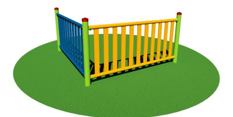
Made entirely of galvanized steel, baked finishing at 180°C. Each module has a length of 200 cm and consists of one round tubular post Ø 89 mm and of one panel made of n°2 horizontal tubular rails Ø50 mm and n°11 vertical tubular picket pales section 80x20 mm. The fence is supplied in an assembly kit, including 1 end post.
