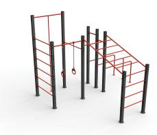
Structure made by poles galvanized steel painted in oven. Tube bars of Ø30 mm. Baked painted steel, with anti-slip finish. Ropes Ø16 mm. reinforced with stainless steel core. Polyethylene rings 20 mm. Safety post caps, anti- vandals. Assembly system with galvanized steel bolts. Fixing in galvanized steel M12, for anchoring to the ground
