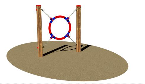
Structure made of Nordic Pine wood pressure treated with non-toxic salts. Components: N°2 glued laminated pine timber poles section cm 7x7 connected through hot dipped galvanized small mesh chains, to a movable hoop in polyethylene PEHD without sharp edges mm 15 thick. Assembly system with 8.8 galvanized steel bolts and self- locking nuts. Coloured nylon cap nuts as required by law. Pole caps in polyethylene.
