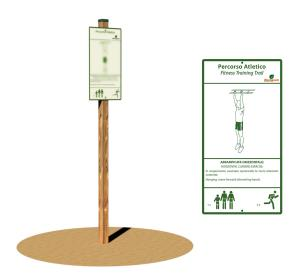
POLE MOUNTED PANEL **To be matched to the Horizontal Climbing exercise fitness trail station - Art. 2123** Aluminium Dibond® panel 62x33 cm, 3 mm thick, that shows how to properly perform the exercise and the number of repetitions. The panel is supported by a pole made of glued laminated pine timber pressure treated with non-toxic salts, section 7x7 cm and 250 cm height, for ground anchoring system.
