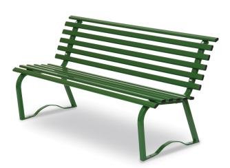
The structure consists of 2 tubular steel supports with a square section 30 x 30 mm with an anatomical shape, 150 cm in length. It consists of twelve steel bars with an oval section 40x20 mm equipped with plastic caps at both ends. Fastening system to the supports through galvanized steel bolts. Anchorage system: to be fixed on the ground. Supplied in an assembly-kit. Entirely galvanized, powder coating at 180°C. Weight:
