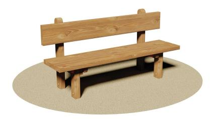
Wooden children's bench. Certificate in accordance with European Standards EN 1176 by the German TÜV - SÜD. Made of pine wood impregnated with non-toxic salts in autoclave. Frame consists of bands section 7x4,5 cm and cross section of reinforcement 7x7 cm. The seat is made up of juxtaposed bands of sect. 9x3,5 cm and the back with strips of sect. 14x3,5 cm. Assembled by 8.8 galvanized steel bolts and nuts. Elements covernut under colored nylon.
