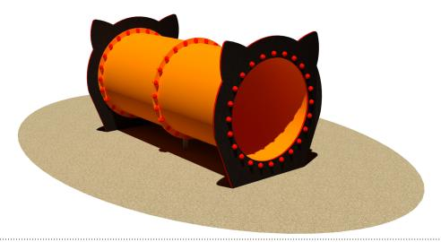
Structure made of 2 circular cylindrical parts realized in fiberglass with high-density multiple coloured layers of resin and 2 decorative panels, as entry and exit point, in multi-layer birch wood glued with phenol formaldehyde resin with non-slip knurled surface and finished with a coloured overlay film in both sides. Assembly system with 8.8 galvanized steel bolts and self- locking nuts. Coloured nylon cap nuts as required by law.
