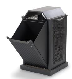
Malta outdoor litter bin. Main structure made of tubular steel, for ground anchoring system. It is equipped with a roof top made of pressed steel sheet, fixed to the structure through 4 stainless steel bolts. Side panels in pressed perforated steel sheet with reinforced edges. Basket in steel sheet with small inner crossbars for attaching the waste bag. Emptying system by unhooking and tilting through hinges. Locking system with key (supplied). Fully galvanized. Powder coating at 180°C.
