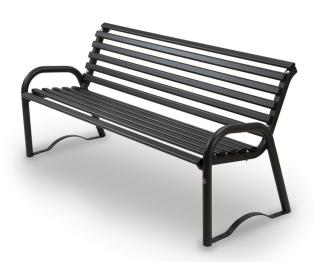
Bologna Bench. Street furniture. The structure consists of 2 tubular steel supports  $\emptyset$  40 mm, with an anatomical shape and with armrests, 158 cm in length. It consists of twelve steel bars with an oval section 40x20 mm equipped with plastic caps at both ends. Fastening system to the supports through galvanized steel bolts. Anchorage system: to be fixed on the ground. Supplied in an assembly-kit. Entirely galvanized, powder coating at 180°C.
