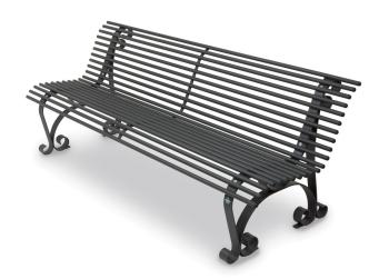
Nostalgia Bench. Outdoor Steel Bench. The structure consists of 2 supports in flat iron shaped bar; 200 cm length. No.22 round steel tubes Ø20 mm, each equipped with plastic caps on either end. Fastening system to the supports through galvanized steel bolts. Anchorage system: to be fixed on the ground. Supplied in an assembly-kit. Colour: micaceous dark grey. Entirely galvanized and baked finishing at 180°C.
