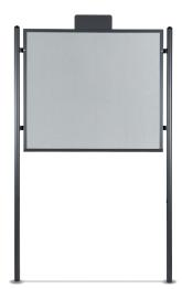
Composed of No. 2 uprights in galvanized steel tubing, Ø 60 mm section, complete with flat iron fittings for the connection of the backboard, made with a galvanized steel tube frame type "1A", section 38x25 mm, and 10/10 galvanized steel sheet. At the top of the backboard, a 20/10 thick galvanized steel plate is positioned for optional customization.
