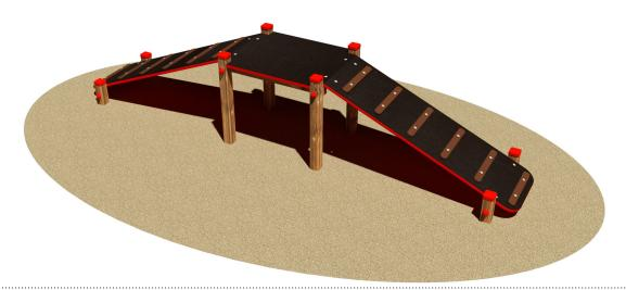
Structure made of Nordic Pine wood pressure treated with non-toxic salts. Components: N°1 horizontal ramp and N°2 inclined ramps in multi-layer birch wood glued with phenol formaldehyde resin with non-slip knurled surface and finished with a coloured overlay film in both sides. The platforms are supported by N°4 glued laminated pine timber poles section cm 7x7. Assembly system with 8.8 galvanized steel bolts and self- locking nuts. Coloured nylon cap nuts as required by law.
