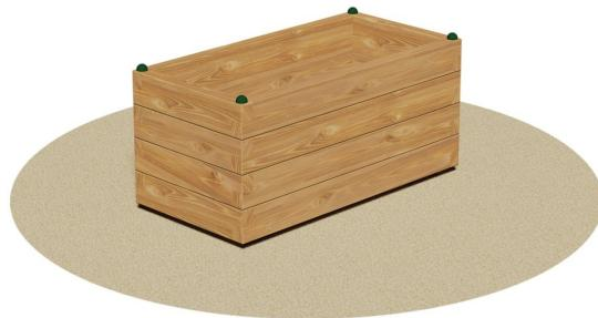
Entirely manufactured with pressure-treated Nordic pine boards, section 11 x 4.5 cm, and base in phenolic-bonded birch plywood with colored film coating on both sides, thickness 1.9 cm. All components are assembled using galvanized steel bolts. The planter is supplied to the Customer in assembly kit form.
