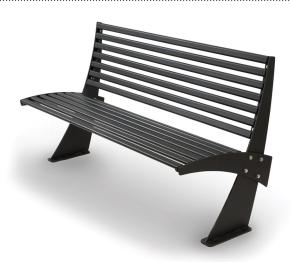
Contemporary bench for street furniture. The structure consists of 2 supports in steel sheet 8 mm thick, with an anatomical shape. The seat and the backrest are composed of 2 units which consist of seven tubular steel bars each with an oval section 40x20 mm. Fastening to the supports through galvanized steel bolts. Anchorage system: to be fixed on the ground. Supplied in an assembly-kit. Entirely galvanized, powder coating at 180°C.
