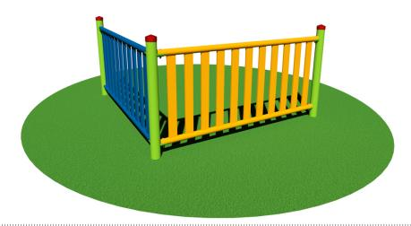
Made entirely of galvanized steel, baked finishing at  $180^{\circ}$ C. Each module has a length of 200 cm and consists of one round tubular post Ø 89 mm and of one panel made of  $n^{\circ}$ 2 horizontal tubular rails Ø50 mm and  $n^{\circ}$ 11 vertical tubular picket pales section 80x20 mm. The fence is supplied in an assembly kit, including 1 end post.
