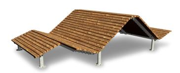
Each module is composed of a tubular steel frame, section 50x30 mm and of flat iron, section 50x8 mm entirely hot-dip galvanized and assembled with Nordic pine wood planks pressure treated, section 60x30 mm. The modules are assembled together by forming two deckchairs, one on each side, with leg support. Supplied in an assembly kit with galvanized steel bolts. Anchorage system: to be fixed on the ground.
