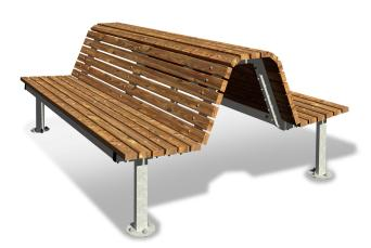
Each module is composed of a tubular steel frame, section 50x30 mm and of flat iron, section 50x8 mm entirely hot-dip galvanized and assembled with Nordic pine wood planks pressure treated, section 60x30 mm. The modules are assembled together by forming two classic seats, one on each side. Supplied in an assembly kit with galvanized steel bolts. Anchorage system: to be fixed on the ground.
